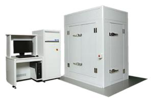
AES biggest advantages are the great surface sensitivity and the high data acquisition speed. PHI 710 guarantees a real nano-scale AES analysis on the sample which has very small features..
