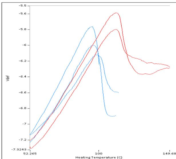
Fig 2. Localized thermal scans resulting from the visibly clear (blue) and the fisheye defect (red) regions of the uncured resin after B-stage. The higher softening transition of the defective region is attributed to a phase rich in diamine curing agent.
