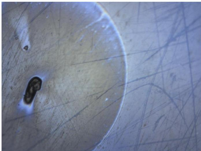
Fig 1. Optical micrograph of the fisheye defect after the coating is cured in an oven.
