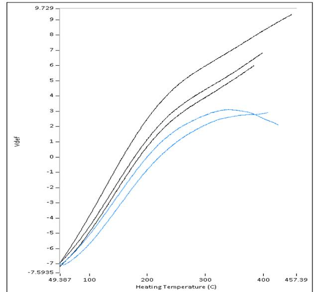
Fig 3. Localized thermal scans resulting from the clear (black) and defective (blue) regions of the film in the cured state. The diamine rich defect does not cure to the same extent.
