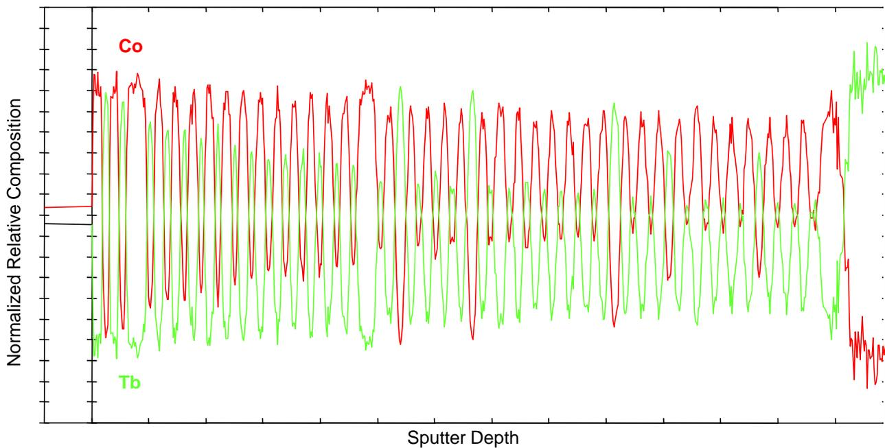
Figure 4. 2.0 kV ion beam energy without Zalar rotation.
