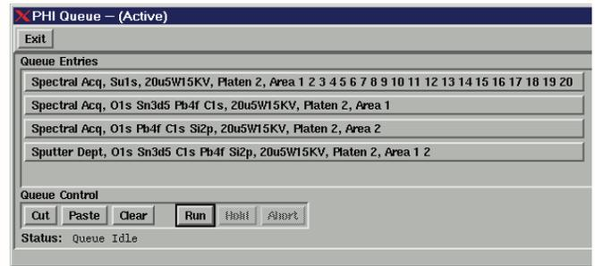
*The Quantera's analysis "Queue" allows multiple analysis tasks to be easily setup for automated analysis*
