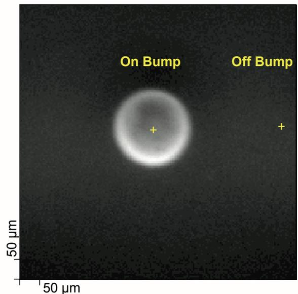
Scanned x-ray beam induced secondary electron image of a solder bump taken by the Quantera SXM
