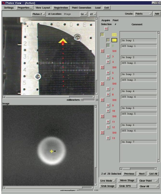
*The Platen View menu provides a point and click interface for analysis area definition from optical, secondary electron and XPS images.*
