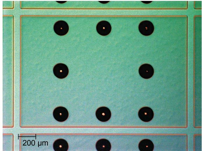
Optical image of solder bumps on a wafer (1072 x 812  $\mu\text{m}$ ) obtained with the Quantera’s sample positioning station
