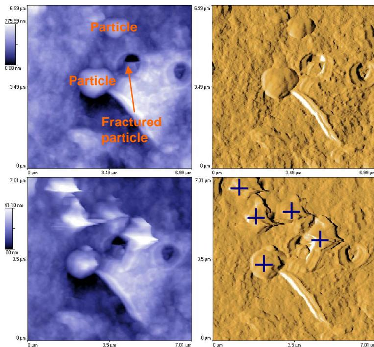
Fig. 2. Cryo-fractured polymer film area 3, 7  $\mu\text{m} \times 7 \mu\text{m}$  AFM topographic and tip deflection images before (top row) and after (bottom row) nano-TA. It is noted that the lateral spatial resolution evident in these images is comparable with that obtained by a conventional AFM probe.
