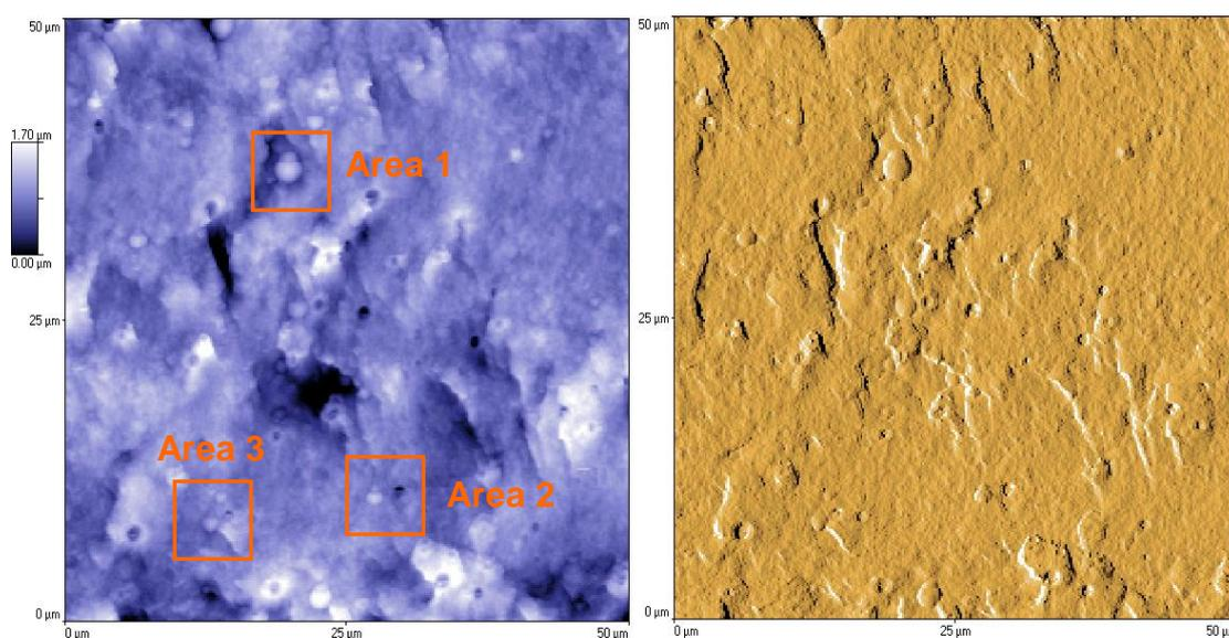
Fig. 1. Cryo-fractured polymer film, 50 μm × 50 μm AFM topographic (left – blue) and tip deflection (right – gold) images. The three marked areas were selected for further imaging and analysis.
