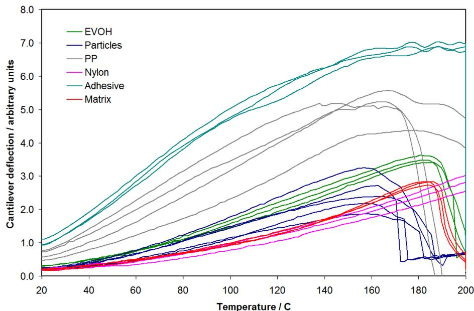
Fig. 5. Overlay of selected nano-TA results from polymer film matrix and all four feedstock materials.
