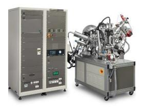
XPS the surface sensitive technique can generally obtain information on elements within a few nms of the sample surface.
